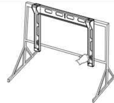
Figure 3.11 Mark the position for hole
