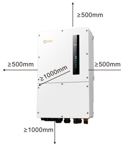
Figure 3.5 Inverter Mounting Clearances
