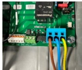
Single Phase Wiring
