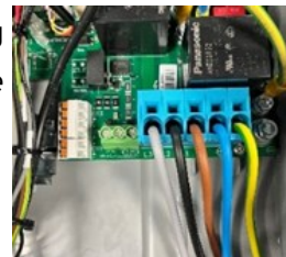
Three Phase Wiring
